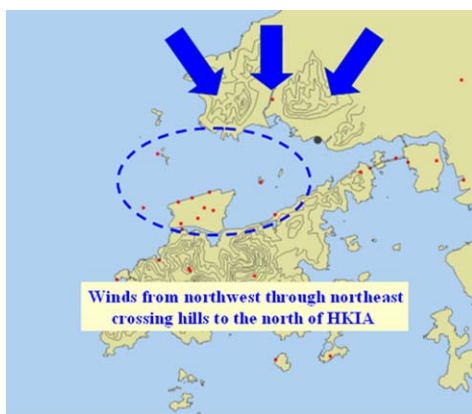
Fig.3c Terrain-induced windshear due to wind flow disturbed by mountains to the northeast of HKIA.
