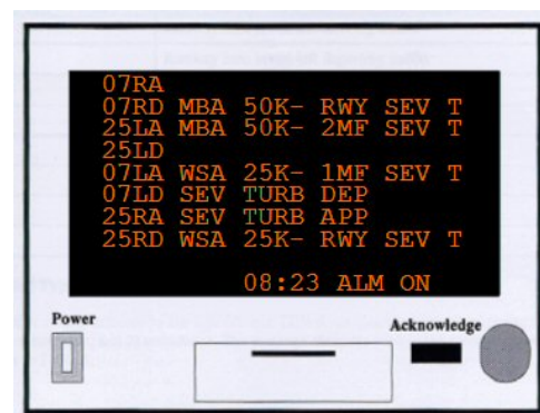
Fig.12b The WTWS Alphanumeric Alert Display installed at the Airport Control Tower showing the windshear and turbulence alerts over various runway corridors at HKIA.
