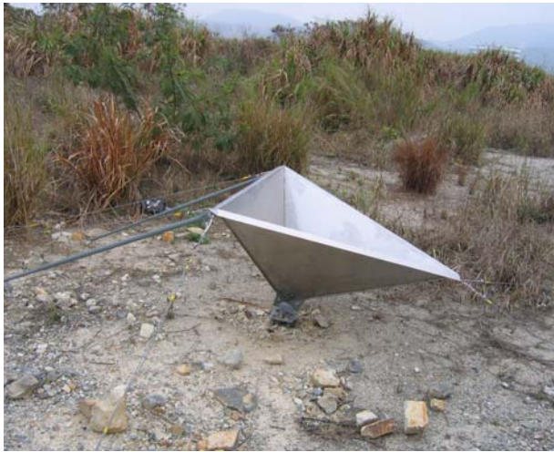
Figure 17 – Corner reflector in Tseung Kwan O
