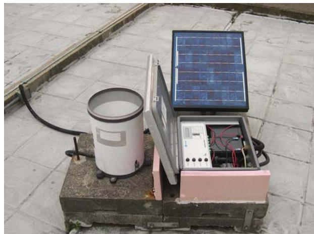
Figure 3 – Typical set up of a raingauge station
